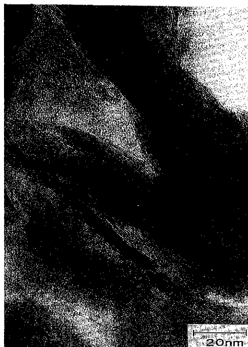
Fig.10 TEM photograph of molybdenum sulfide comminuted in n-decane containing oleic condition : before HCl treatment
