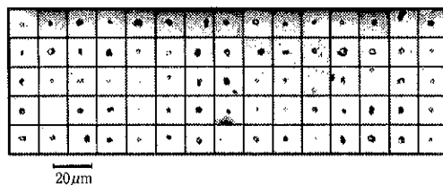
Fig.6 Observed images of agglomerates in class-6, prepared by dispersing WA# 6000 particles in 0.05wt.% sodium hexametaphosphate solution
