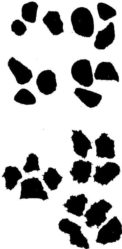
Fig. 2 Sand shapes (9-12mesh) top Original below Plastic-coated
