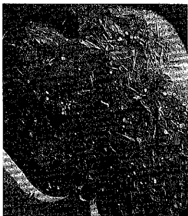
Fig. 7. Electron micrograph of surface structure of the particles in the flyash by two-stage self-molding replica method.
