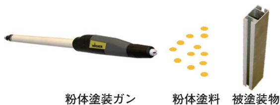
図3 粉体塗装部分の構成 Fig. 3 Arrangement of the powder painting parts.
