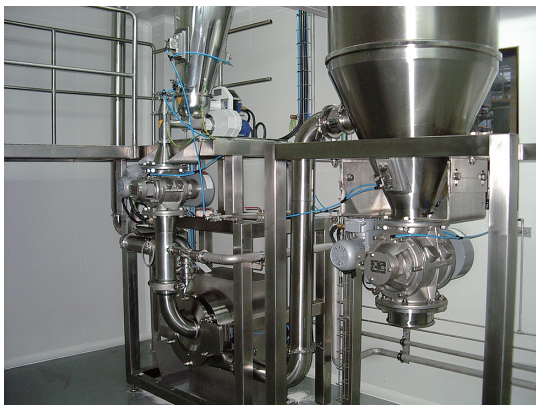
図7 PSR (Pressure shock resistance) 10bar仕様の微粉碎UPZ Fig. 7 Fine grinding mill UPZ of PSR (Pressure shock resistance) 10bar specification
