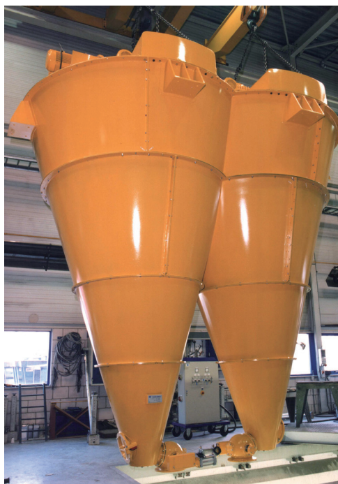
Fig. 3 Double cone execution of the Nauta Mixer, a double cone efficiently doubled the working volume of the blender without adding additional height.
