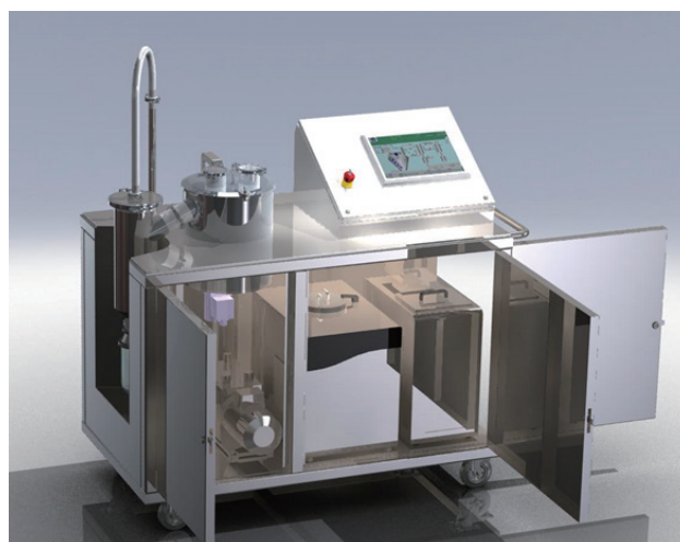
Fig. 7 Laboratory AFD unit. Including controls, vacuum system, freeze condenser and heating/cooling unit.
