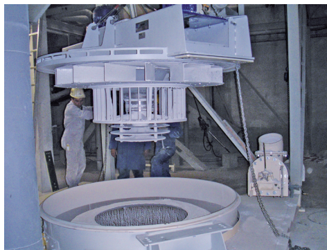
Fig. 10 Section drawing of Ventoplex C and dismantling of a C21V
