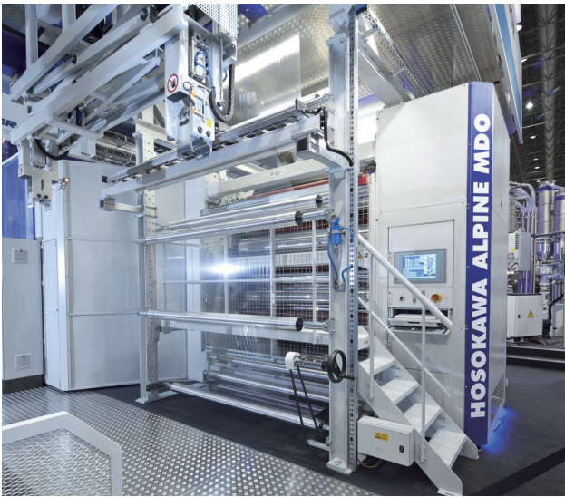
Fig. 20 Mono-axial film orientation line MDO
